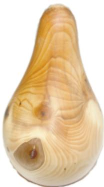
Ron rounded over the end and cut the indentation found in the top of an apple. He then drilled a hole for the stalk. After turning most of the apple shape, Ron
