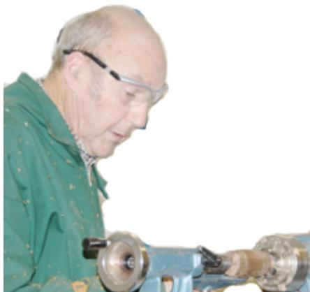
Ron started with a Yew blank, 3" square and 8" long. This was enough for an apple and a pear. After rounding over the top of the pear, Ron drilled a hole in the end for the stalk. Ron then used a spindle gouge to shape the pear, followed by sanding, sealing, buffing and parting off.
