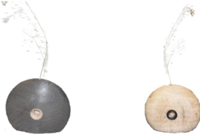
Mark's final piece was another vase from a single 1" x 6" board. As before, he mounted the board on a screw chuck and turned the edge to round. Mark then hollowed the centre, leaving a flat 1/8" rim. Reversing the piece, Mark turned the outside to a saucer shaped curve. He removed it from the chuck and cut it in half, before gluing the halves together to form the vase.
