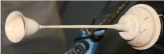
At this point, Mark used a parting tool to define the captive ring. Using the roughing gouge and spindle gouge to remove material either side of the
