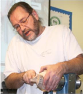
Mark's project was a three-legged vessel in Oak. Mounting the blank between a step drive centre and a ring centre, he used a spindle roughing gouge to true up the piece. This was followed by a long grind bowl gouge to rough out the shape. Mark cut a parallel chucking spigot at the tail-stock end and reduced the diameter of the section where the legs would appear. The blank was then mounted in a chuck. Mark squared off the end with a normal grind gouge and made a small
