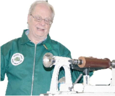
Stan's project for the evening was an open bines vase in mahogany (from an old newel post). Mounting the blank between steb centres, Stan cut a chucking spigot with a parting tool and created a dovetail using a skew chisel. He then mounted in the chuck and brought up the tail stock for support. Stan turned the blank to a cylinder and squared off the end.
