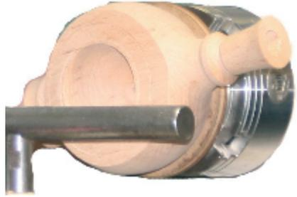
As a contrast, the two bungs are made from a different coloured wood. Holding the bung blank between a scrap of wood covered by router mat, and the live centre, Paul first cut a spigot to fit into the hole in the body. He then mounted the bung in the chuck and turned several beads to decorate the outside. Paul uses melamine lacquer and carnuba wax as a finish.
