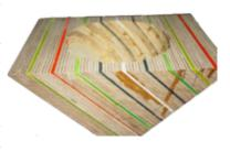
MDF ring over the top of the bowl. This will be turned away as late as possible. Wearing a glove to protect his hand, Dennis hollows the inside first using a Simon Hope tungsten carbide tipped tool. He uses a circle template to get the perfect round shape on the inside. This is indicated by a "bullseye" in the plywood rings.
