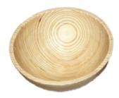
A teardrop scraper smoothes the inside. Dennis rough sands the inside and then coats it with Isaac Lord's Mitre adhesive (a type of superglue). This supports the wood fibres allowing a second use of the scraper to produce a finer finish. Another coat of superglue is sanded to 1000 grit to produce a glossy finish. The bowl is parted off and reverse chucked to
