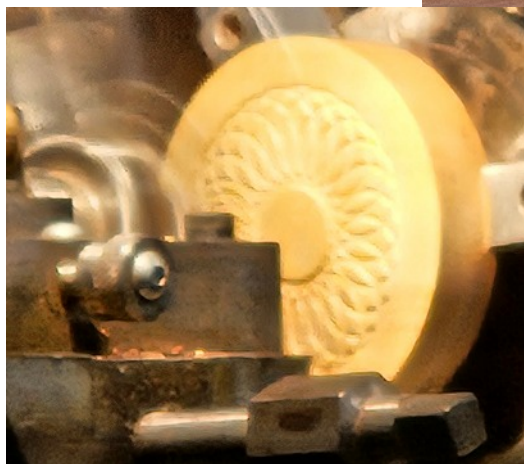
Above & Right: Cutting a pattern into wood e.g. The top of a box.
